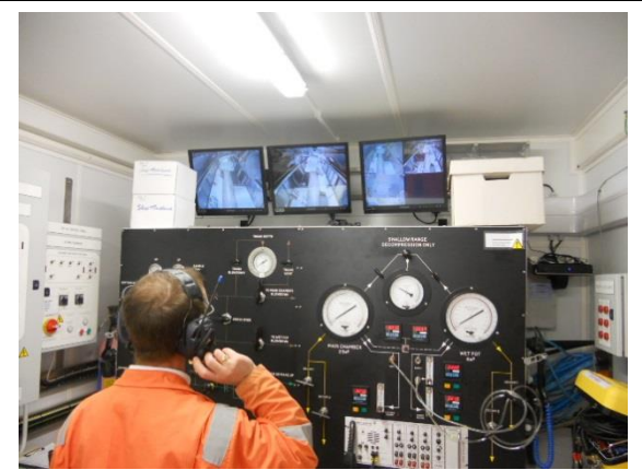
Inside the BP Baku HRF saturation control cabin with the Supervisor communicating with and watching the divers inside the HRF.
