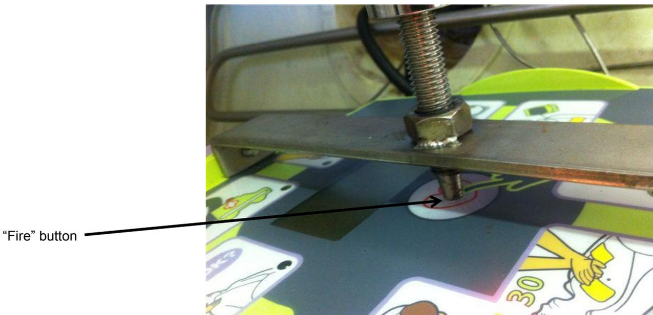
Figure 5. Screw drive activation of AED Plus
