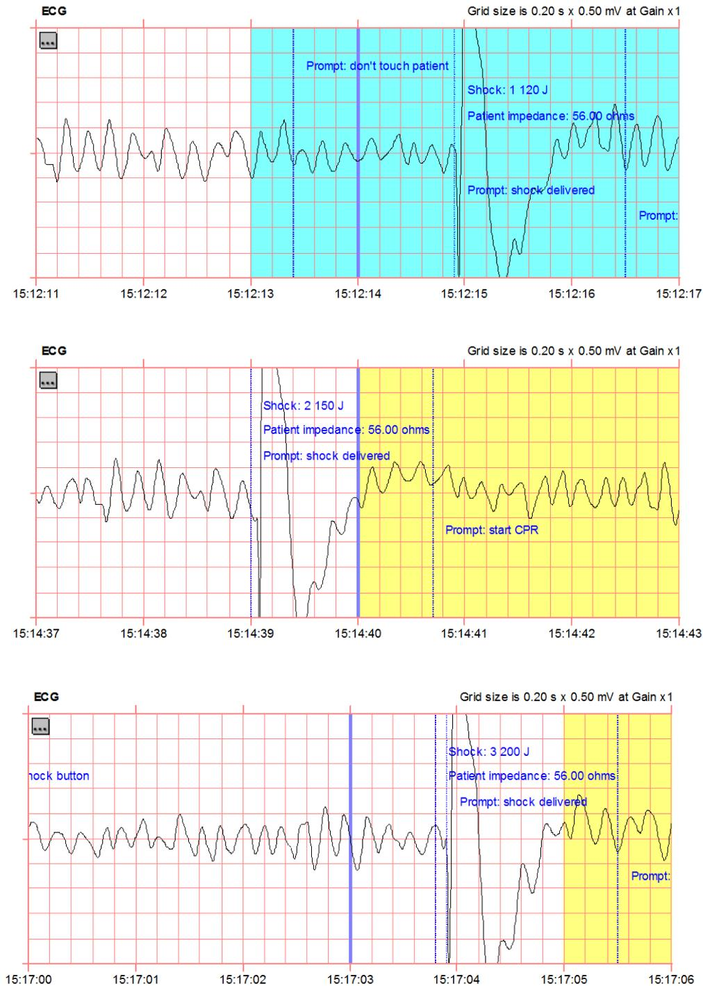
Figure 13. Extracts from downloaded data showing shock delivery through penetrator on chamber 3 on Seawell
