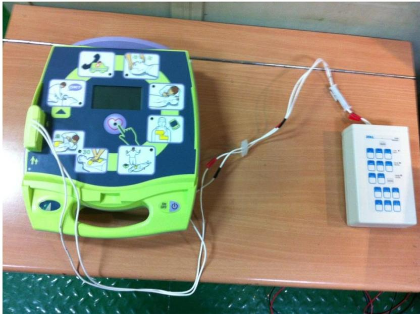
Figure 14. Defibrillator connected to ECG simulator.
